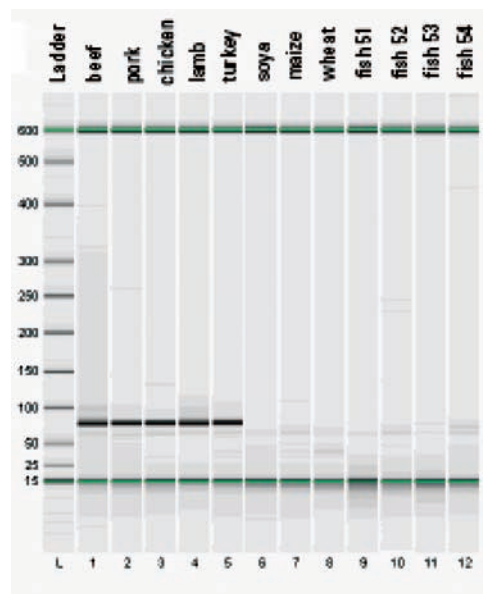
Figure 4. Agilent 2100 Bioanalyzer gel-like image showing PCR test designed to discriminate meat. Positive results are evident in lanes 1 through 5 for various meat products. Lanes 6 through 12 show negative results for grain and fish.
